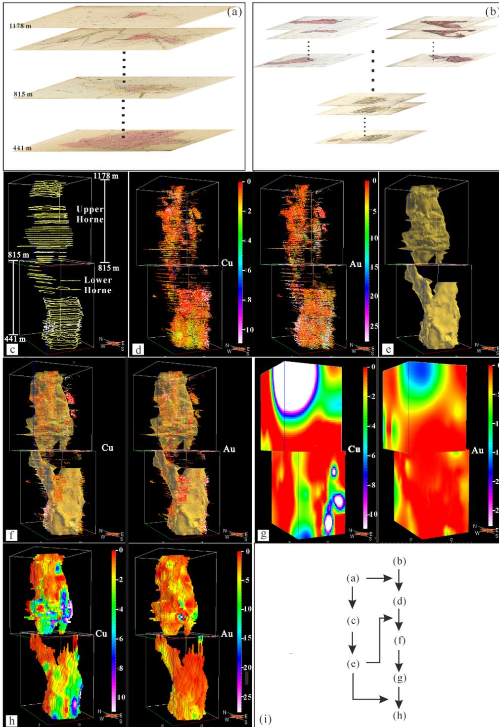
( a ) Level plans; ( b ) stopes; ( c ) outlines of each elevation; ( d ) assay data of each elevation; ( e ) orebody surface; ( f ) block of surface and assay data; ( g ) initial 3D block model; ( h ) 3D block model and assay value distribution of Au and Cu; ( i ) flow chart of 3D model construction. The reference plane ( 0 m ) of the model in Fig. 4 is 1 178 m as shown in Fig. 3 and the area of 441–1 178 m in Fig. 4 is the area of 737–0 m shown in Fig. 3.
